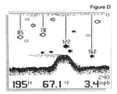
Figure D shows a view with "Small Digits" selected in the User Options menu. By selecting smaller digits for the depth, speed and temp information, more of the screen is available for the graphic representation of the sonar information. This effectively increases the display resolution of the Wide 2000, allowing targets which are very close together to be displayed as separate symbols.
